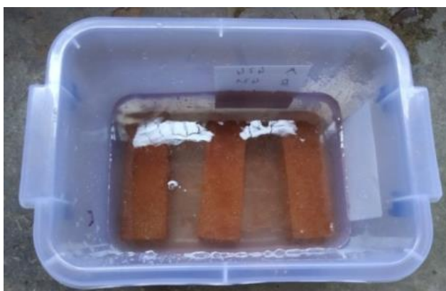
Figure 2 : Water resistance test by immersion
